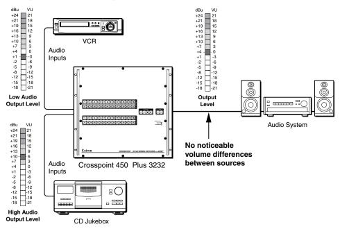
Figure 3-56 — Audio gain and attenuation
